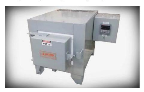
Lucifer Furnaces recently announced it has supplied a bench style box furnace to Lycian Stage Lighting, a manufacturer of theatrical followspot lights. The model HA7-A9 has chamber dimensions of 6 x 6 x 9 in. and heats to 1,850°F. Temperature is controlled with a Honeywell microprocessor-based digital time proportioning controller with accuracy of 0.25%.
