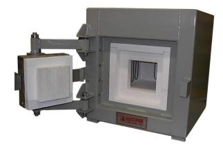
High temperature furnaces equipped with molybdenum disilicide heating elements and alumina ceramic fiber insulation for rapid heat to 2700°F, 2900°F or 3100°F. Compact lightweight design and low power requirements make these models ideal for R&D, Industry, and Schools for processing ceramics, precious metals and composite materials.
