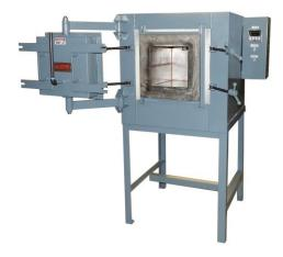
Bench and floor models equipped with an alloy muffle for operation with a positive flow of protective atmosphere to 2050°F. The alloy muffle separates the chamber refractory and heating elements from the workload and atmosphere to minimize scale and oxidation on most tool steels. This design achieves lower dew points, reduces atmosphere consumption and shortens purge time. The AM models are ideal for cyclical or production type applications.
