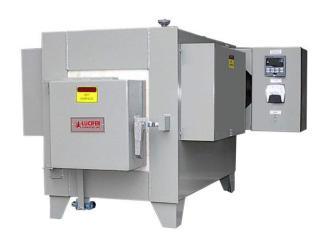
The EHS3 models are a low cost alternative for processing high speed steels and ceramics with operation to 2450°F. Ideal for Tool & Die shops, Laboratories and Schools. Equipped with silicon carbide heating elements mounted across the roof and lightweight ceramic fiber insulation forming a compact energy efficient package. Designed with an SCR power supply to automatically regulate the voltage for changes in the element resistance and workloads providing optimum performance at the lowest cost.
